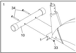
While another person lifts the back of the Frame (1), attach the Rear Stabilizer (28) to the Frame with two M10 x 75mm Carriage Bolts (34) and two M10 Nylon Locknuts (33).
